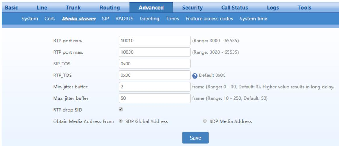
**Figure 2-31 MX60/MX60E/MX120G Media Stream Configuration Interface**
