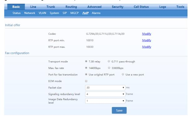
Figure 2-12 MX60/MX60E/MX120G Fax Configuration Interface
