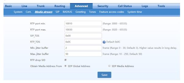
Figure 2-31 MX60/MX60E/MX120G Media Stream Configuration Interface
