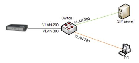
1. Configure multi-service VLAN on the HX4 device: the voice VLAN uses mode 1, the VLAN tag is 300, the VLAN tag of the management VLAN is 200, and the IP address is obtained from the corresponding VLAN network using DHCP. As shown in Figure 3-10.
