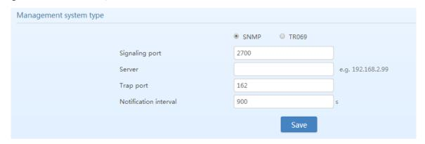
**Table 2-25 SNMP Configuration Parameters**
